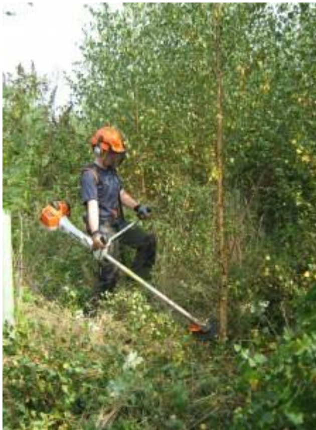
Picture 3.7 shows a brush saw in use. These are especially efficient for cutting stems with diameter smaller than 8 cm. The equipment could however be used for bigger stems, but the efficiency compared to a chain saw significantly drop when the average diameter exceeds 8 cm.
